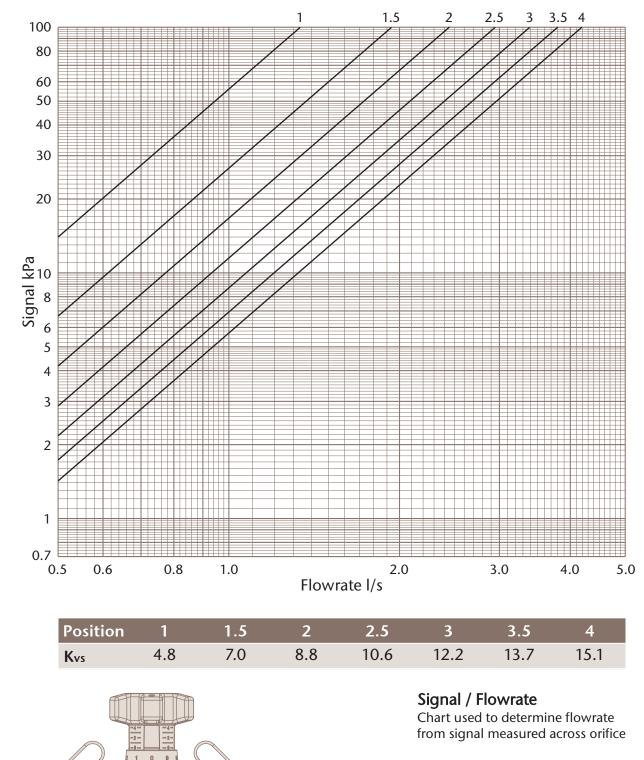
$Q = \frac{K_{VS} \sqrt{\Delta p}}{36}$ Where  $Q = Flowrate \qquad l/s$   $\Delta p = Signal \qquad kPa$   $K_{VS} = Signal Co-efficient$
